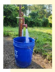
Flow rate is a measure of the quantity of water that flows over a given time period and is measured in gallons per minute (GPM) and gallons per hour (GPH). A simple way to determine flow rate is to place a 5-gallon pail beneath your water source, open the valve completely, and count how many seconds it takes to fill the pail.
